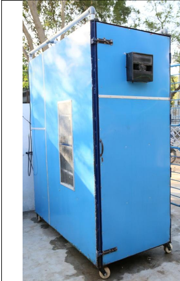
Low Cost Hydroponic Device (40 kg/Day production capacity) produced by the influence of the scheme
